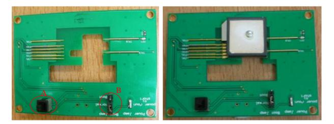
As shown in upper photos. Area "A" is the power switch. The power is ON when the toggle switch is at lower position. On the contrary, the power is OFF when the toggle switch is at higher position.
