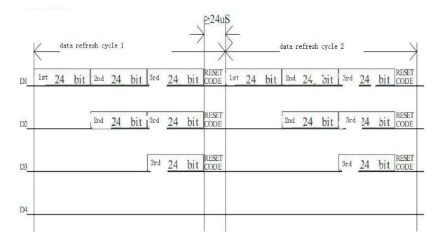
Note:D1 send data for MCU side,D2、D3、D4 forward the data for automatically shaping of cascade TM1804.
