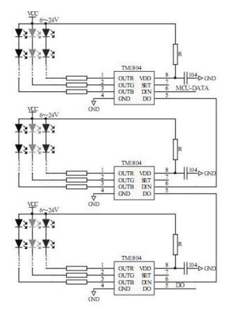
The TM1804 can confirgurate to6-24v Voltage for power supply,but according the input voltage is different,it should configurate different power resistant, the resistance is as bellow:
