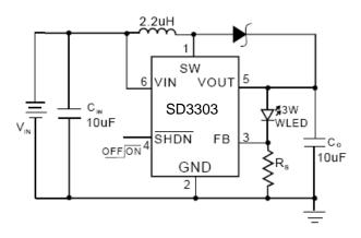
$I_{LED} = 750 \text{mA}, R_S = 0.127 \Omega$
