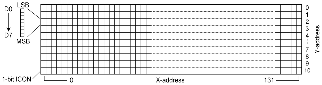
Figure 14 RAM format and addressing, if DO=0
