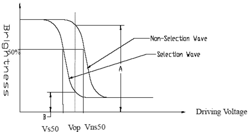
Contrast Ratio =  $\frac{\text{Brightness of Non-Selected condition (A)}}{\text{Brightness of Selected condition (B)}}$
