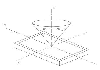
Inspection should be performed within angle ( is usually 30°) from Z axis to each X and Y.
