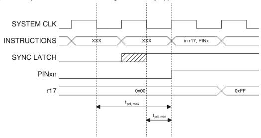
Consider the clock period starting shortly *after* the first falling edge of the system clock. The latch is closed when the clock is low, and goes transparent when the clock is high, as indicated by the shaded region of the "SYNC LATCH" signal. The signal value is latched when the system clock
