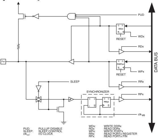
Note: 1. WPx, WDx, RRx, RPx, and RDx are common to all pins within the same port.  $clk_{I/O}$ , SLEEP, and PUD are common to all ports
