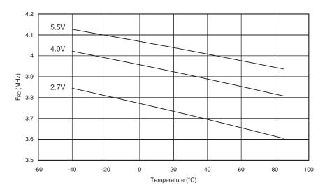
Figure 174. Calibrated 4MHz RC Oscillator Frequency vs.  $V_{\rm CC}$
