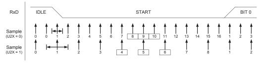
When the clock recovery logic detects a high (idle) to low (start) transition on the RxD line, the start bit detection sequence is initiated. Let sample 1 denote the first zero-sample as shown in
