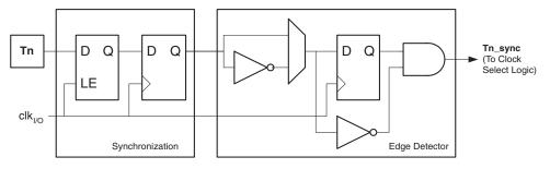
The synchronization and edge detector logic introduces a delay of 2.5 to 3.5 system clock cycles from an edge has been applied to the T1/T0 pin to the counter is updated.
