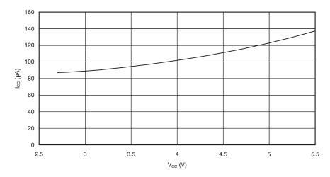
Figure 142. Standby Supply Current vs.  $V_{CC}$  (6MHz Xtal, Watchdog Timer Disabled)
