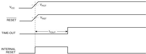
Figure 16. MCU Start-up, RESET Extended Externally
