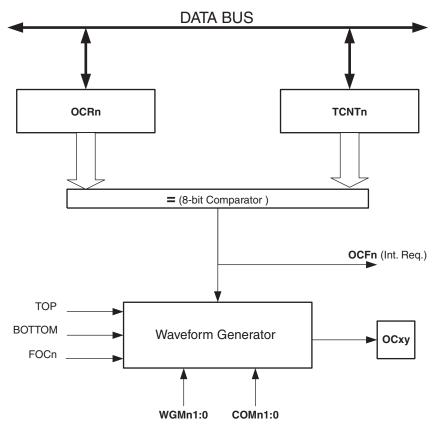
The OCR2 Register is double buffered when using any of the Pulse Width Modulation (PWM) modes. For the normal and Clear Timer on Compare (CTC) modes of operation, the double buffering is disabled. The double buffering synchronizes the update of the OCR2 Compare Register to either top or bottom of the counting sequence. The synchronization prevents the occurrence of odd-length, non-symmetrical PWM pulses, thereby making the output glitch-free.
