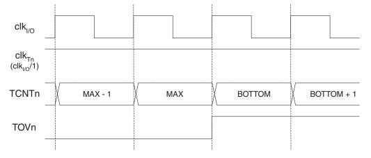
Figure 53 shows the same timing data, but with the prescaler enabled.
