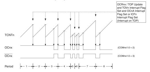
The Timer/Counter Overflow Flag (TOV1) is set each time the counter reaches TOP. In addition the OCF1A or ICF1 Flag is set at the same timer clock cycle as TOV1 is set when either OCR1A or ICR1 is used for defining the TOP value. If one of the interrupts are enabled, the interrupt handler routine can be used for updating the TOP and compare values.
