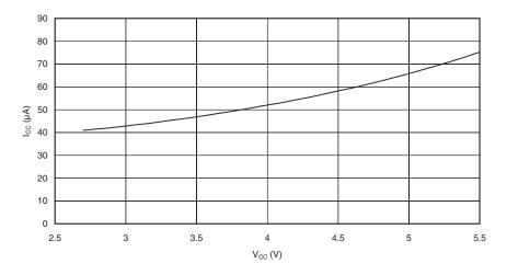
Figure 138. Standby Supply Current vs. V<sub>CC</sub> (2MHz Xtal, Watchdog Timer Disabled)
