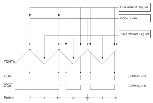
Figure 51. Phase Correct PWM Mode, Timing Diagram
