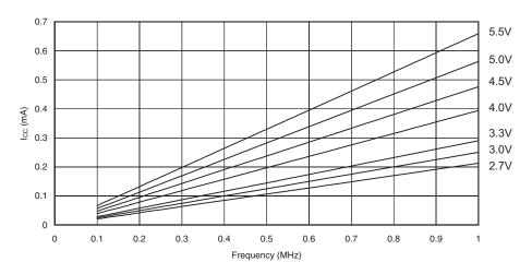
Figure 126. Idle Supply Current vs. Frequency (1MHz - 20MHz)
