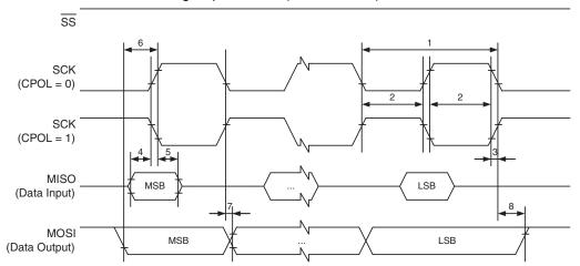
Figure 117. SPI interface timing requirements (Slave Mode)
