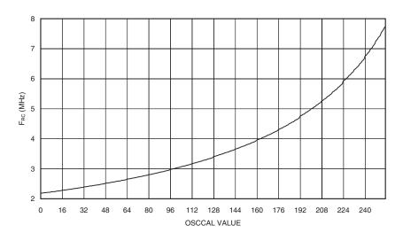
Figure 175. Calibrated 4MHz RC Oscillator Frequency vs. Osccal Value
