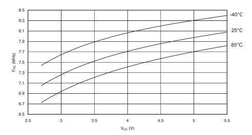
Figure 171. Calibrated 8MHz RC Oscillator Frequency vs.  $V_{\rm CC}$
