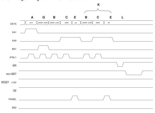
Figure 107. Programming the EEPROM Waveforms
