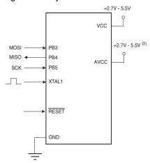
Notes: 1. If the device is clocked by the Internal Oscillator, it is no need to connect a clock source to the XTAL1 pin
