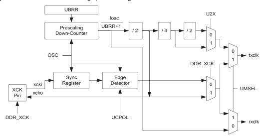
Figure 62. Clock Generation Logic, Block Diagram
