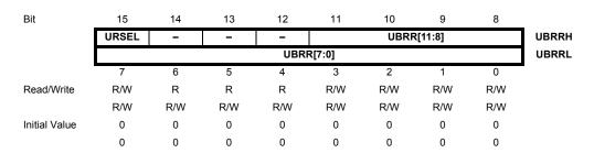
The UBRRH Register shares the same I/O location as the UCSRC Register. See the "Accessing UBRRH/UCSRC Registers" on page 146 section which describes how to access this register.
