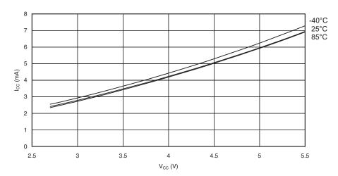
Figure 127. Idle Supply Current vs.  $V_{\text{CC}}$  (Internal RC Oscillator, 8MHz)
