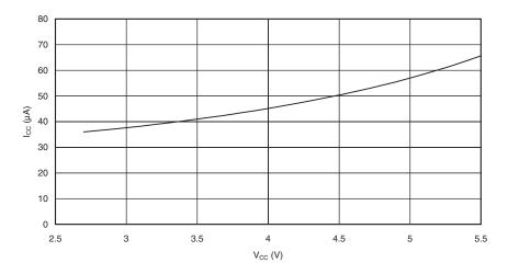
Figure 136. Standby Supply Current vs. V<sub>CC</sub> (1MHz Resonator, Watchdog Timer Disabled)
