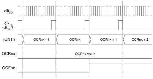
Figure 43 on page 95 shows the count sequence close to TOP in various modes. When using phase and frequency correct PWM mode the OCR1x Register is updated at BOTTOM. The tim-
