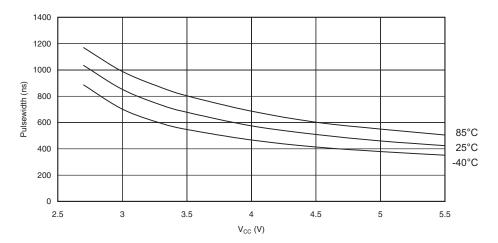
Figure 191. Reset Pulse Width vs.  $V_{\text{CC}}$
