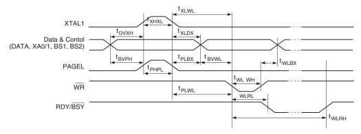
Figure 110. Parallel Programming Timing, Loading Sequence with Timing Requirements<sup>(1)</sup>
