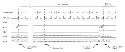
Figure 93. ADC Timing Diagram, Single Conversion
