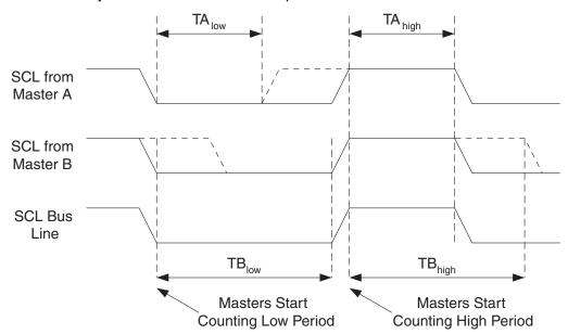
Figure 74. SCL Synchronization Between Multiple Masters
