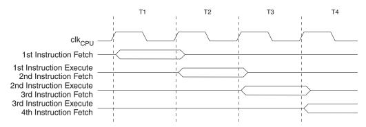
Figure 6 shows the internal timing concept for the Register File. In a single clock cycle an ALU operation using two register operands is executed, and the result is stored back to the destination register.
