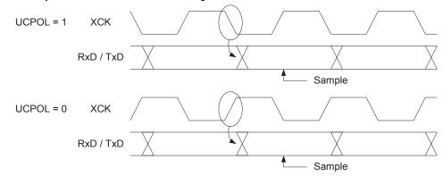
The UCPOL bit UCRSC selects which XCK clock edge is used for data sampling and which is used for data change. As Figure 63 shows, when UCPOL is zero the data will be changed at rising XCK edge and sampled at falling XCK edge. If UCPOL is set, the data will be changed at falling XCK edge and sampled at rising XCK edge.
