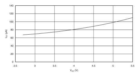
Figure 139. Standby Supply Current vs. V<sub>CC</sub> (4MHz Resonator, Watchdog Timer Disabled)
