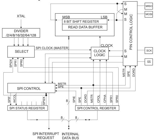
Note: 1. Refer to "Pin Configurations" on page 2, and Table 22 on page 58 for SPI pin placement
