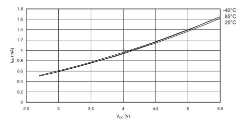
Figure 130. Idle Supply Current vs.  $V_{\text{CC}}$  (Internal RC Oscillator, 1MHz)
