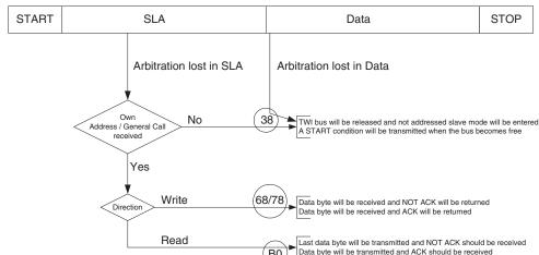
Figure 88. Possible Status Codes Caused by Arbitration
