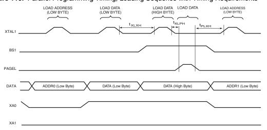
Note: 1. The timing requirements shown in Figure 109 (that is, t<sub>DVXH</sub>, t<sub>XHXL</sub>, and t<sub>XLDX</sub>) also apply to loading operation
