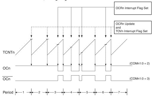
The Timer/Counter Overflow Flag (TOV2) is set each time the counter reaches MAX. If the interrupt is enabled, the interrupt handler routine can be used for updating the compare value.
