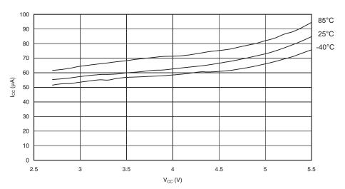
Figure 187. Analog Comparator Current vs.  $V_{\text{CC}}$
