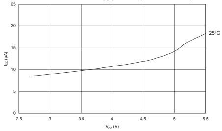
Figure 186. Watchdog Timer Current vs.  $V_{\rm CC}$
