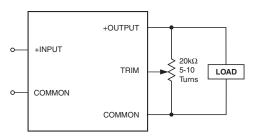
Figure 6. Trim Connections Using a Trimpot
