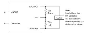
Figure 7. Trim Connections Using Fixed Resistors
