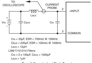
Figure 2. Measuring Input Ripple Current
