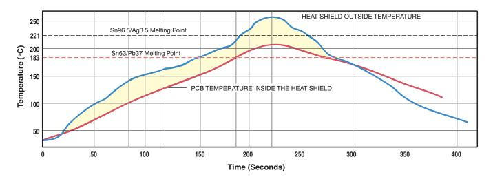
Figure 6. Reflow Solder Profile
