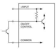
ON/OFF pin open: Logic High = DC/DC converter On ON/OFF pin <0.4V: Logic Low = DC/DC converter Off
