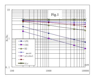
Fig.1 shows the typical sensitivity characteristics of the MQ-4, ordinate means resistance ratio of the sensor (Rs/Ro), abscissa is concentration of gases. Rs means resistance in different gases, Ro means resistance of sensor in 1000ppm Methane. All test are under standard test conditions.
