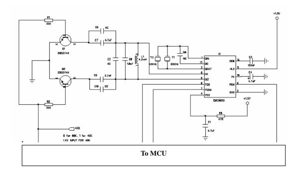
The MCU is responsible for the control of switch between the two frequencies, controlling the power on (PON) of the receiver IC as well as analyzing the pulses that are provided as output from the CME6005 (TCO or TCON)
