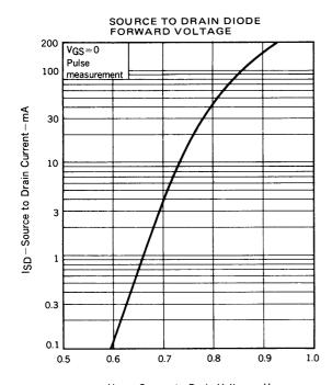
$v_{SD}\!-\!\text{Source to Drain Voltage}\!-\!v$
