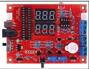
Step 32: Install 1pcs DIP-28 STC15W408AS at U4. Align gap mark on IC and gap mark on DIP-28 IC Socket. They are used to specify the installation direction.
