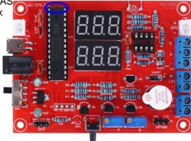
Step 33: Install 1pcs DIP-8 IC LM358P at U3 by the same methods.
