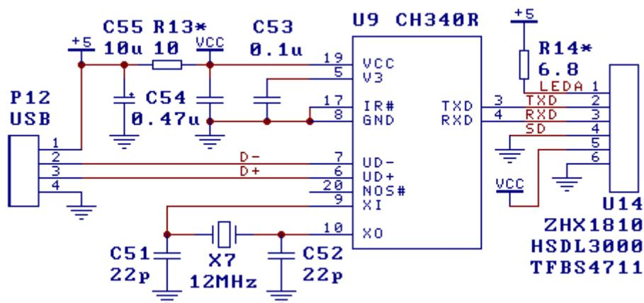
The image above is a USB to infrared adapter design which is composed with USB convert IrDA infrared chip CH340R and infrared transceiver U14 (ZHX1810/HSDL3000 etc). The resistor R13 is used to weaken influence of large current in infrared transmitting. The current limiting resistor R14 should be adjusted according to the manufacturer’s recommended value of the infrared transceiver U14.
