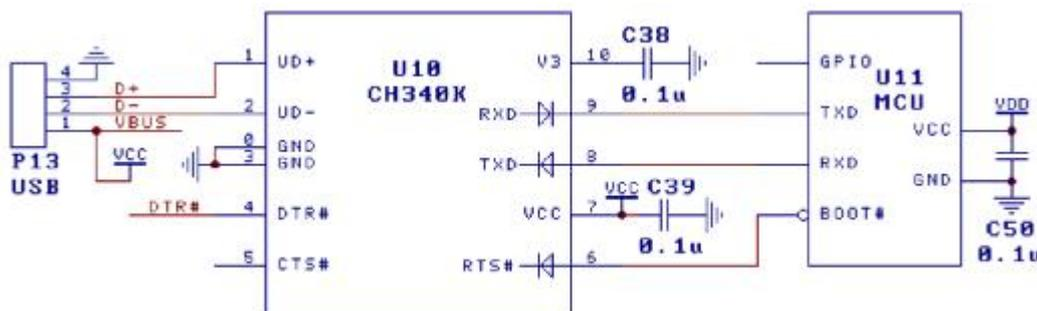
The figure above shows the reference circuit for USB communication between the MCU and the CH340K via UART. CH340K is powered by the USB bus VBUS (VCC), the MCU uses another power supply VDD, which
