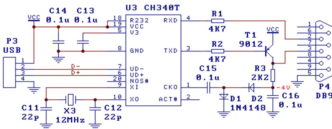
The image above is USB to RS232 converter design too, the function of this circuit is the same with 7.2 section except the range of output RS232 is narrower. When R232 pin is driven high, the assistant RS232 function will be enabled, just need to add some diodes, transistors, resistors and capacitors, the special level conversion chip U5 in section 7.2 could be replaced and the hardware cost is lower.
