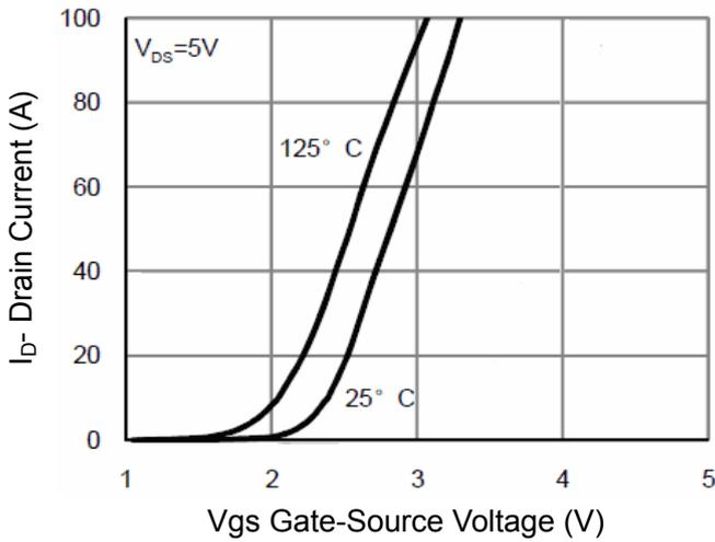
Figure 2 Transfer Characteristics
