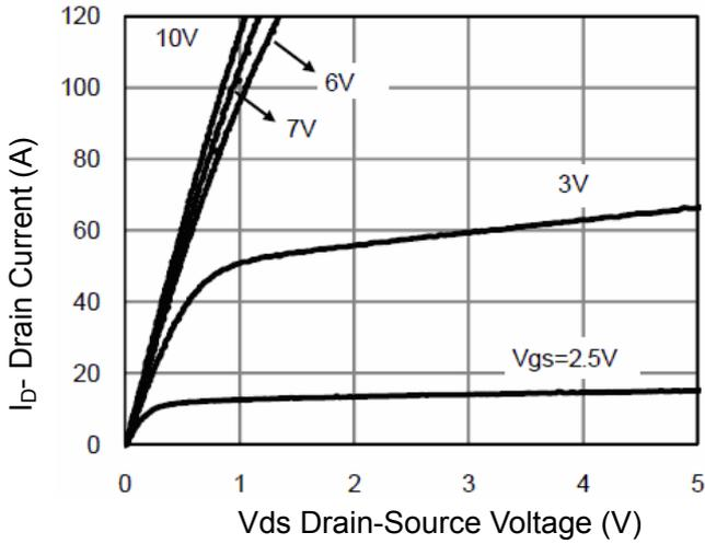
Figure 1 Output Characteristics
